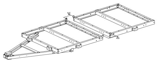
Figure D: Assembling Front and Rear Beds
